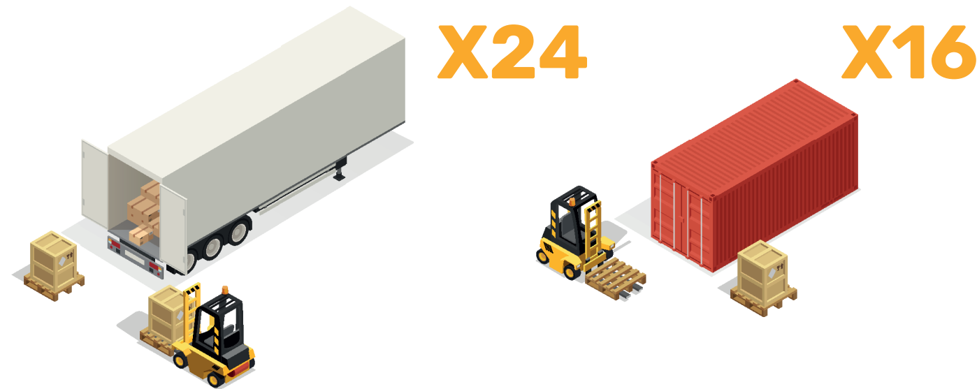
24 Duomods can be transported with an 90m³ truck.
