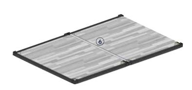
Align the floor coverings and stick floor connection covers
